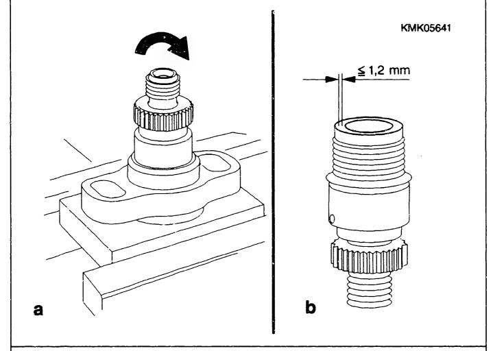
Re-install barrel-and-flange element in line with corresponding pump repair instructions.
